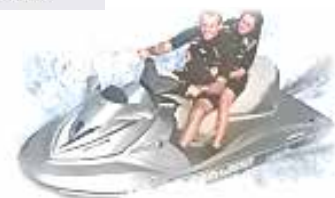
A PWC (Personal Water Craft) has a planing hull
